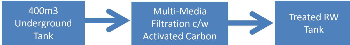
1. Continuing from the Underground RW Tank, it is filtered by a multi media water treatment system.
